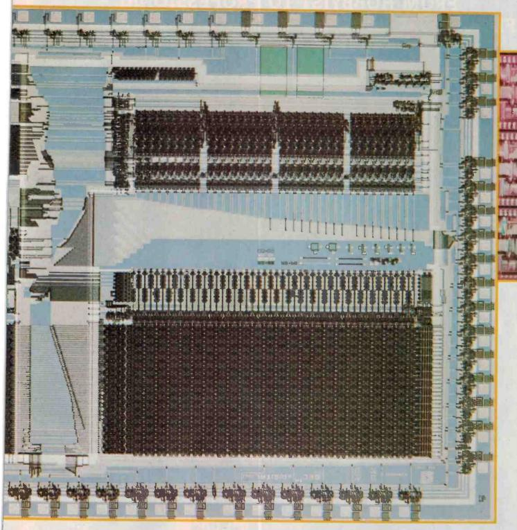
down' order: first the functional design of the system, then design of the logic to perform the required functions, then design of the circuits to perform that logic, and finally the translation of the final circuit into the nitty-gritty geometric patterns and connections etched, diffused and deposited on the chip surface.
