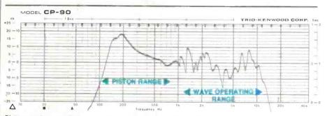
Plstons and waves. Typical response of a low frequency drive unit, showing the piston operating region and the wave operating region.
