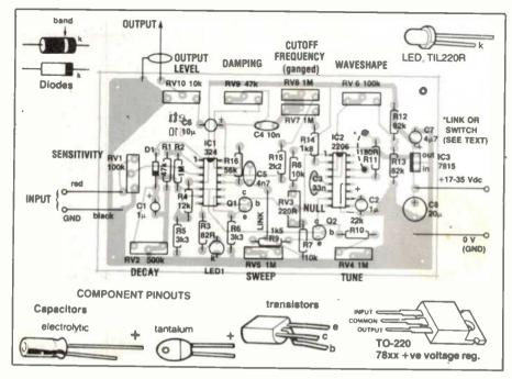
If you are using preset potentiometers for all the variable resistors, it is best to fit them all next. You may wish to use potentiometers, with knobs fitted, for RV2 and RV4 to 10. If so, leave these for the moment.
