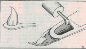
Figure 20. 'Icicles' sometimes form on a joint when you remove the iron. Reheat the joint with a clean iron to get rid of them.
