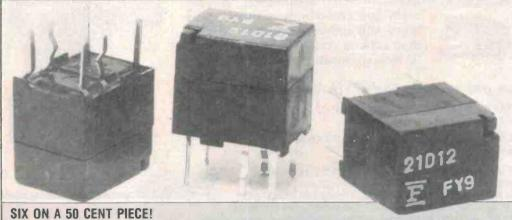
These new Fujitsu FBR20 series miniature relays are small enough that six will comfortably fit on a 50 cent piece! Despite their microminiature size, the SPDT contacts are rated at 1 A/24 Vdc (resistive) or 0.5 A/120 Vdc (resistive).
