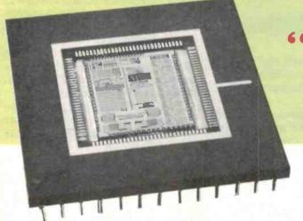
The 102 000-transistor chip, designed and constructed as a design exercise, is a voice recognition device.
