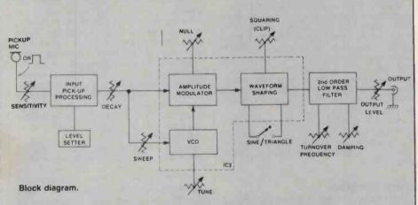
base of Q2. When the input signal exceeds one Vbe drop (about 0.6 V), corresponding to a beat of medium force, Q2 sinks current from pin 7 of IC2. The current drawn out of pin 7 defines the frequency of oscillation of the VCO, so this has the effect of 'sweeping' the tone when the drum is struck in any but the gentlest manner. RV5 allows the degree of sweeping to be set; RV4 clearly sets some basic amount of current out of pin 7, so it has the effect of 'tuning' the drum.
