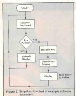
Should a key be pressed, the microprocessor decodes the key and updates the display panel with the new information from the keyboard. The system contains a number of LED display characters, and in a multiplexing scheme, each should be kept on for a specified period of time (in this case 1 ms) before moving to the next character. This example shows in which submodule the system spends most of its time and why.
