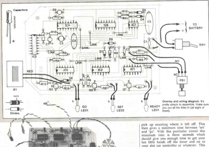
that the circuit is in the 'ready' mode. This LED is lit after the pushbutton is pressed once. It indicated that the circuit is ready for action.
