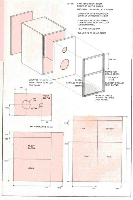
Commence by cutting out the boxes and assembling them, but leave the back panels off for the moment. Screw the speakers in place, placing sealing compound around the rim of each where they meet the front baffle. I oriented each driver so that the terminals faced each other.
