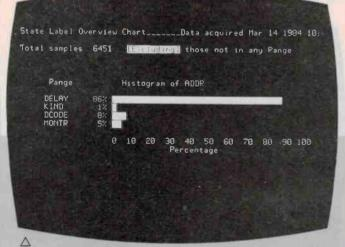
Figure 5. Overview histogram of state activity in monitor, decode, and display modules.
