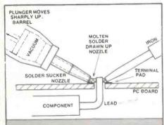
Figure 22. Using a solder sucker. First heat the joint until the solder melts. Then apply the solder sucker nozzle and release the plunger to suck up the molten solder. It is sometimes best to remove the iron before releasing the plunger. The solder sucker's nozzle and barrel has to be cleared of the solid solder 'dags' periodically.
