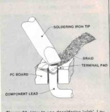
Figure 21. How to use desoldering 'wick'. Lay it over the joint and appaly the iron tip to the braid, using a little pressure. The solder will be drawn into the brald. When this happens, remove the iron and braid. Cut off the used braid.
