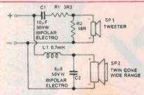
Circuit. Simple, isn't it. Note that the tweeter is connected in the opposite phase to the twin-cone to ensure their outputs add in the crossover region.
