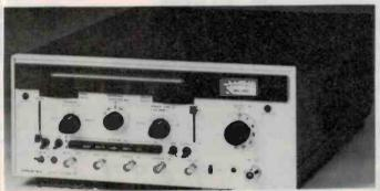
tal-controlled harmonic markers at 1, 10, 50, 100 and 500 MHz intervals as standard equipment. The marker system features dual-amplitude markers for easy identification. In application, the markers may be tilted up to 90° for easy viewing when displayed with steep transition signals.
