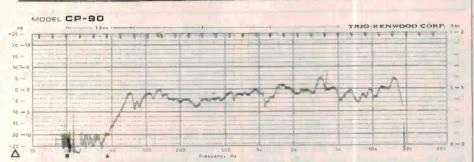
Frequency response. The speakers have a reasonably smooth frequency response (measured on the tweeter axls) with few significant peaks and dips. The bass response will lift somewhat when they're mounted near the floor.
