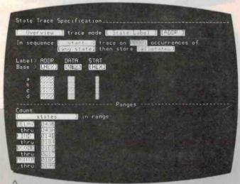
Figure 4. Trace specification for tracing state activity of monitor, decode and display modules.
